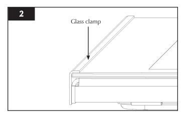
To free glass if sealant has been used, carefully run a sharp knife between the glass and the glass gasket beneath. Always cut away from the body.
